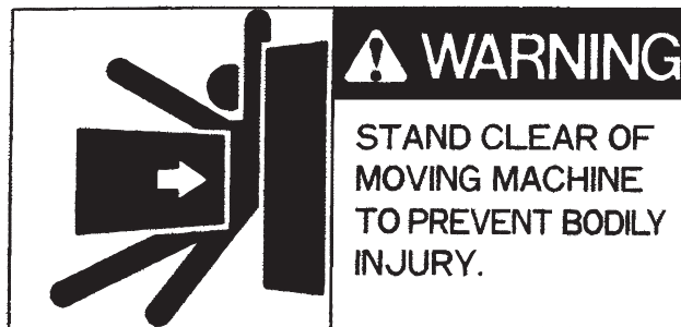
(18) Being crushed by machine
