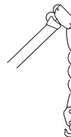
(2) Rope with left-hand turns viewed up from the hook block
