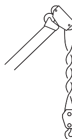
(1) Rope with right-hand turns viewed up from the hook block
