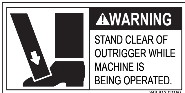
(16) Being crushed by outrigger float
