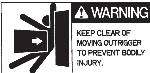
(15) Being crushed by outrigger
