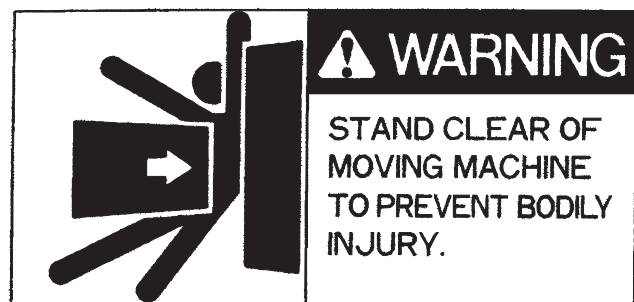
(20) Being crushed by machine
