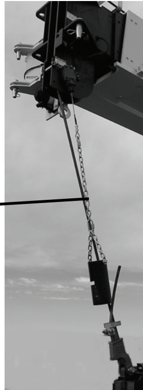
Incorrect ATB Position for Travel ATB Weight and Chain Hanging on ATB Switch
